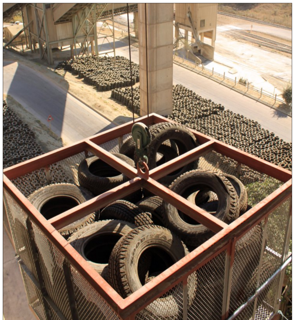
Waste put to good use: Tyres are hoisted up to the testing area during the alternative fuel trials at the NPC-CIMPOR cement plant at Simuma recently. As the picture shows, a vast number of reject and waste tyres can be redeemed as even the trials consumed about 2880 tyres per day.
